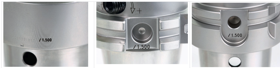
Fig. 4: Marking for checking of the clamping force: Three possible positions on the clamping chuck
